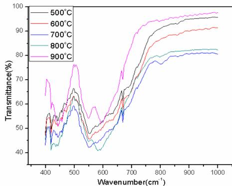
**Fig. 3** FT-IR spectra of  $\text{Sr}_{0.5}\text{La}_{0.5}\text{Mg}_{0.5}\text{Fe}_{11.5}\text{O}_{19}$  ferrite particles.
