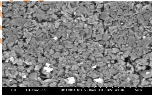
**Fig .2** SEM Morphology  $\text{Sr}_{0.5}\text{La}_{0.5}\text{Mg}_{0.5}\text{Fe}_{11.5}\text{O}_{19}$  ferrite(a) heated at 600 °C and (b) heated at 900 °C
