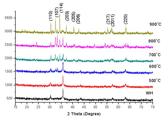
**Fig 1.** X-ray diffraction patterns of  $Sr_{0.5}La_{0.5}Mg_{0.5}Fe_{11.5}O_{19}$  ferrite at different annealing temperature.
